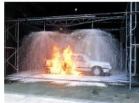
Foam Extinguishing Test
