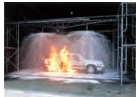
Foam Extinguishing Test
