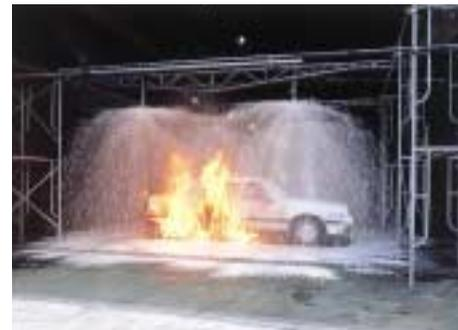
Foam Extinguishing Test
