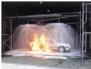
Foam Extinguishing Test
