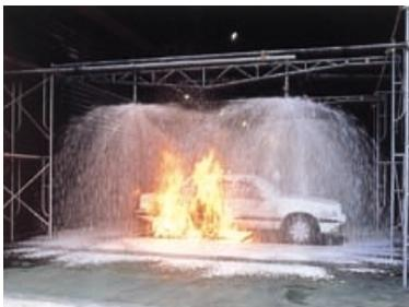
Foam Extinguishing Test
