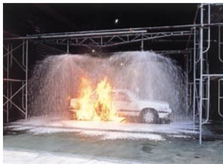
Foam Extinguishing Test
