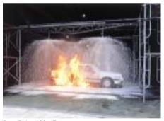
Foam Extinguishing Test
