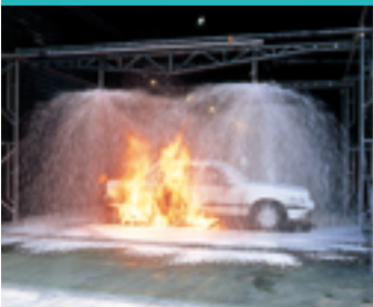
Foam Extinguishing Test
