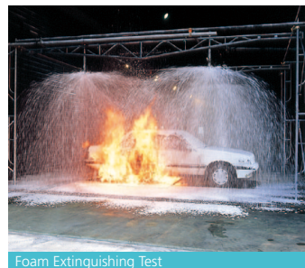
Foam Extinguishing Test
