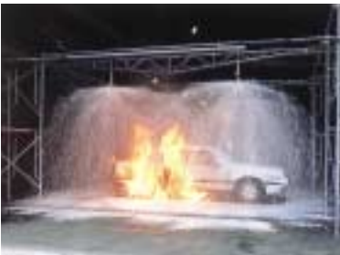
Foam Extinguishing Test
