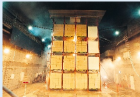
Rack warehouse fire test
