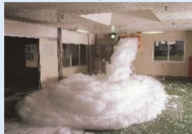
Foam fire extinguishing test
