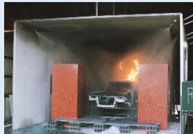
Automotive paint booth fire test
