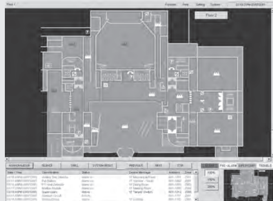
Floor plan under alarm condition
