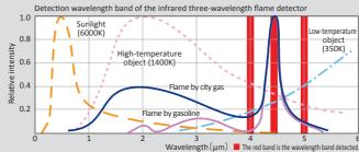
The infrared energy emitted from flames has the spectral characteristics of a peak in the wavelength of the 4.4u
