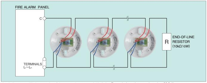
ullet Lead wire system ullet Maximum number of detectors to be connected : No limit. ullet External wire resistance : Less than  $50\,\Omega/\text{line}$
